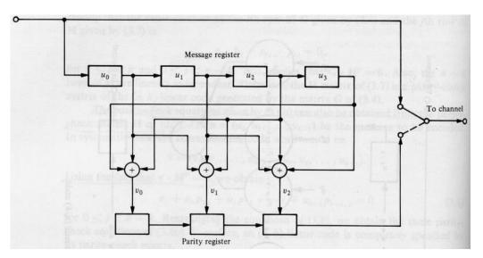
Figure: Encoding Circuit for (7,4) code
