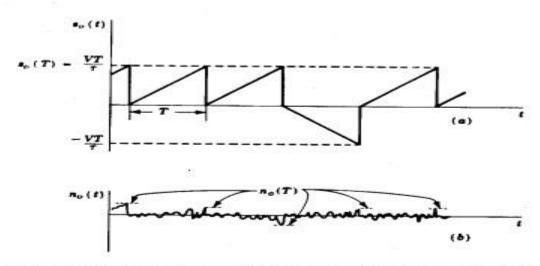
Figure 11.1-3 (a) The signal output and (b) the noise output of the integrator of Fig. 11.1-2.
