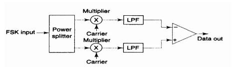
FIGURE 2-8 Coherent FSK demodulator
