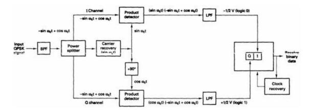
FIGURE 2-21 QPSK receiver
