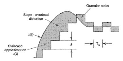
Fig. Quantization errors in delta modulation
