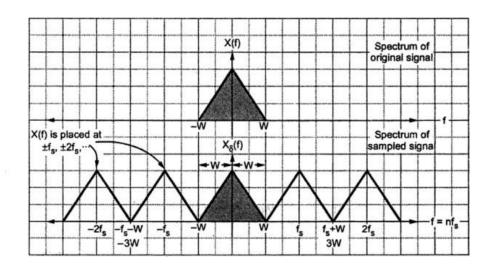
Fig. 6 Spectrum of original signal and sampled signal
