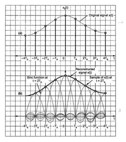
Fig. 7 (a) Sampled version of signal x(t) (b) Reconstruction of x(t) from its samples
