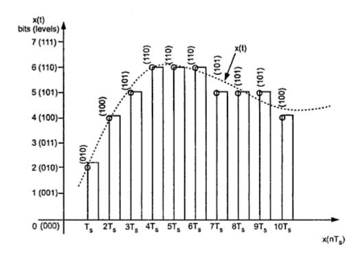
Fig. Redundant information in PCM
