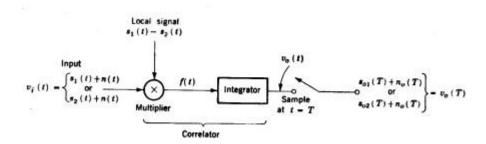
Fig:11.6-1 Coherent system of signal reception
