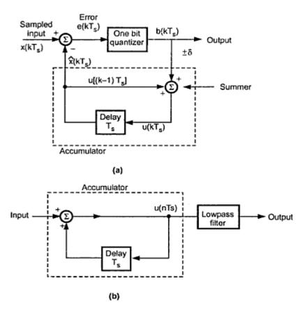
Fig. (a) Delta modulation transmitter and (b) Delta modulation receiver
