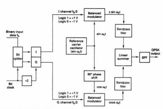
FIGURE 2-17 QPSK modulator
