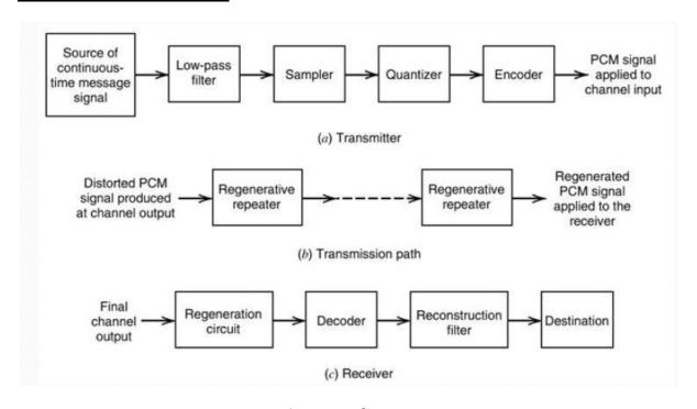
Fig. 3 Elements of PCM System
