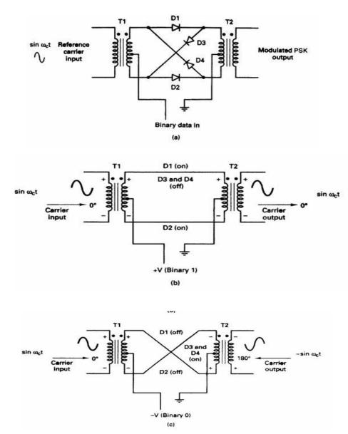
FIGURE 9-13 (a) Balanced ring modulator; (b) logic 1 input; (c) logic 0 input
