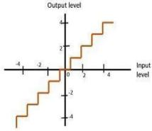
Fig 2 : Mid-Tread type Uniform Quantization
