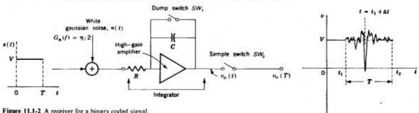
Figure 11.1-2 A receiver for a binary coded signal.
