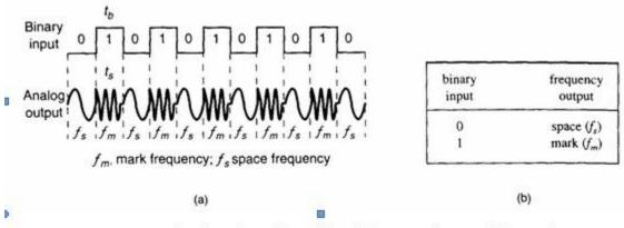
FIGURE 2-4 FSK in the time domain: (a) waveform: (b) truth table
