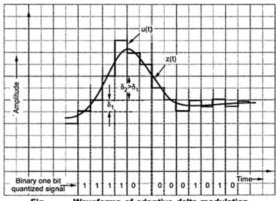
Fig. Waveforms of adaptive delta modulation
