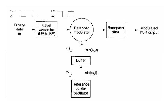
**FIGURE 2-12 BPSK transmitter**
