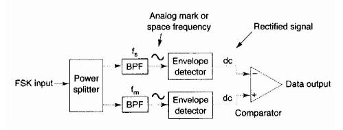
FIGURE 2-7 Noncoherent FSK demodulator
