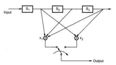
Fig. 4.4.32 Convolutional encoder of example 4.4.8
