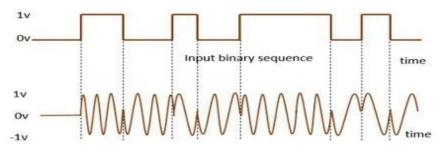
BPSK Modulated output wave
