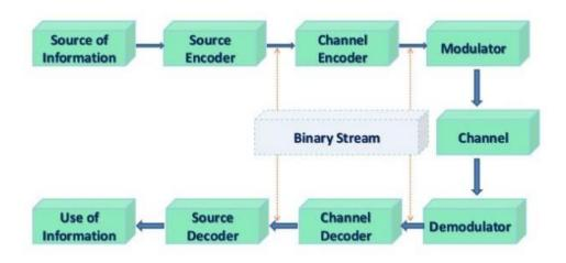
Fig. 1 Elements of Digital Communication Systems
