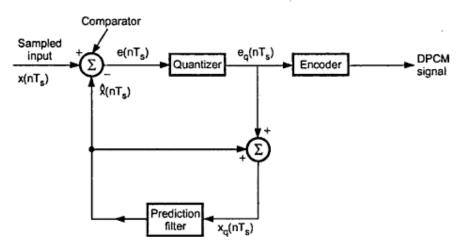
Fig. Differential pulse code modulation transmitter
