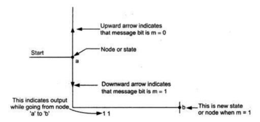
Fig. 4.4.5 Code tree from node 'a' to 'b'
