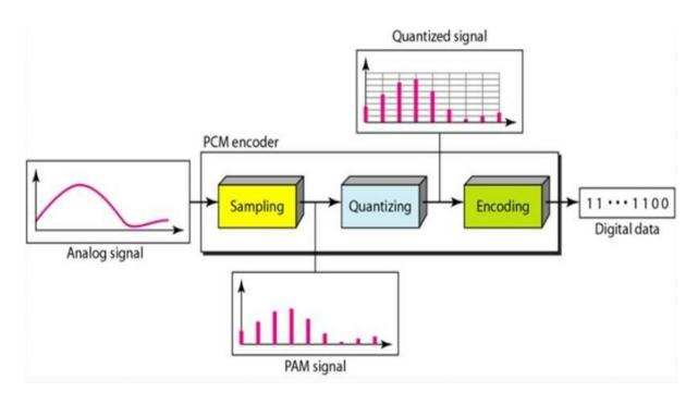
Fig. 2 Conversion of Analog Signal to Digital Signal
