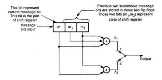
Fig. 4.4.4 Convolutional encoder with k = 1 and n = 2
