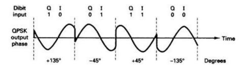
FIGURE 2-19 Output phase-versus-time relationship for a PSK modulator
