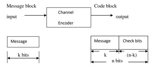
Figure: Functional block diagram of block coder
