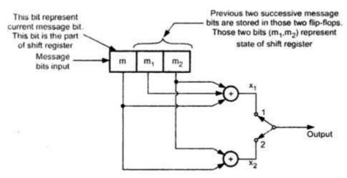
Fig. 4.4.1 Convolutional encoder with k = 3, k = 1 and n = 2
