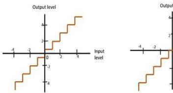
Fig 1: Mid-Rise type Uniform Quantization
