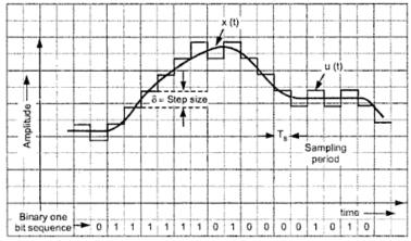
Fig. Delta modulation waveform
