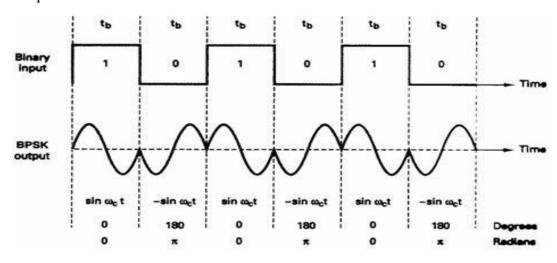
FIGURE 2-15 Output phase-versus-time relationship for a BPSK modulator
