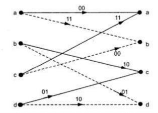
Fig. 4.4.34 Code trellis diagram for steady state
